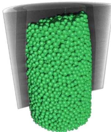
*3D reconstruction of the glass beads test sample, voxel size  $(4.5 \mu\text{m})^3$ , 1000 projections, 12 s scan duration, ORYX FLIR camera, "1x" Hasselblad lens*
