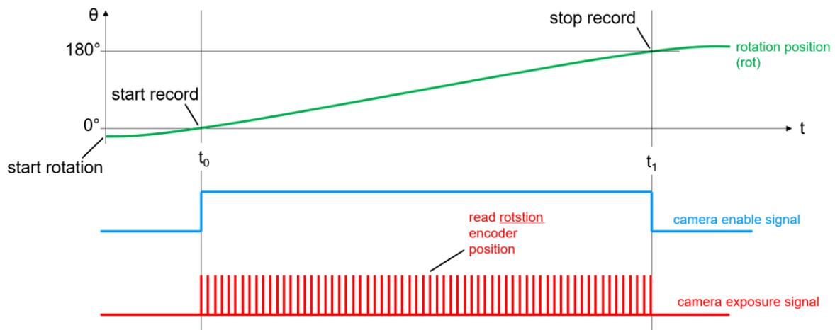
In this mode, the rotation of the sample is set to a constant angular velocity, while the camera continuously acquires projections, each image stored with the corresponding reading of the rotation encoder. This is the standard, fast scanning modality.
