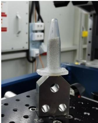
*Test sample glass beads: The glass spheres in their sample holder mounted on the BEATS tomography sample stage*
