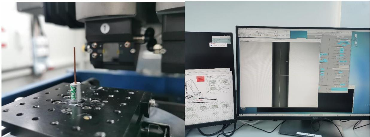
*Alignment of the Nb<sub>3</sub>Sn superconducting wire sample*
