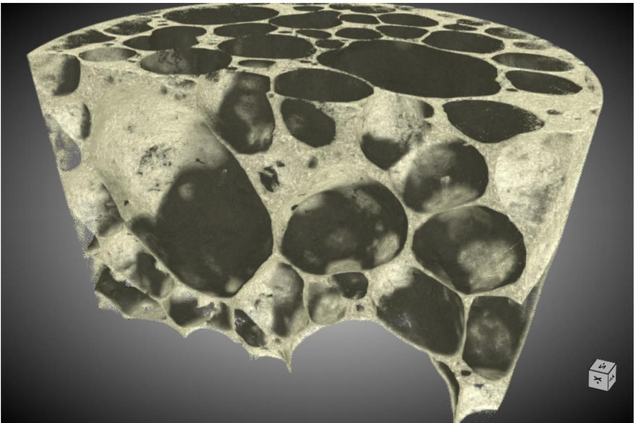
*Al foam, 3D reconstruction, voxel size (6.5  $\mu\text{m}$ )<sup>3</sup>*
