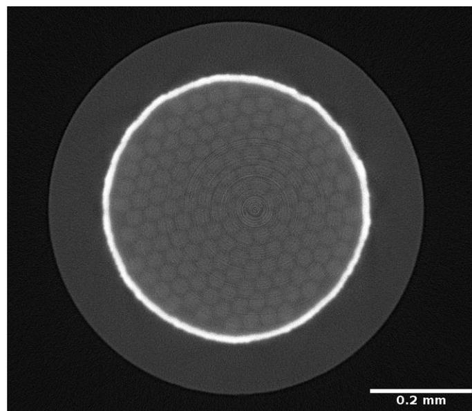
*Nb<sub>3</sub>Sn superconducting wire, slice of the 3D reconstruction*
