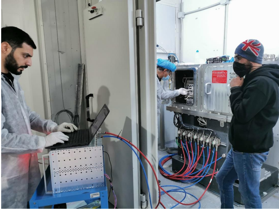
The DMM installed at the Optics Hutch of BEATS at SESAME during the motion axes test
